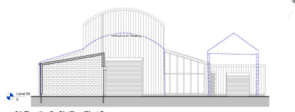
GA Elevation D - Distillery/Plant Room 1:100
